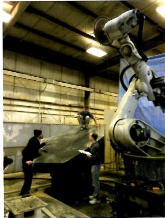
Figure 1.8 Stone fabrication involved the precise subtraction of materials from the rough cut quarry block. A combination of saws, CNC machines, and robotic machines removed material from the blocks to the exact geometry of the memorial units.
